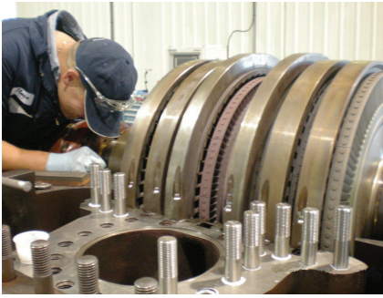
Checking seal clearances during re-assembly.
